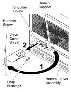
Figure 17 - Removing Valve Cover Shield
